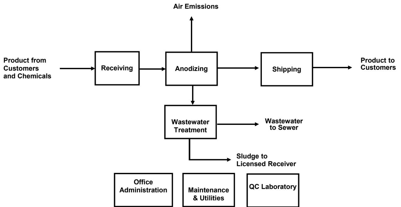
Anodizing Process Flow Diagram
