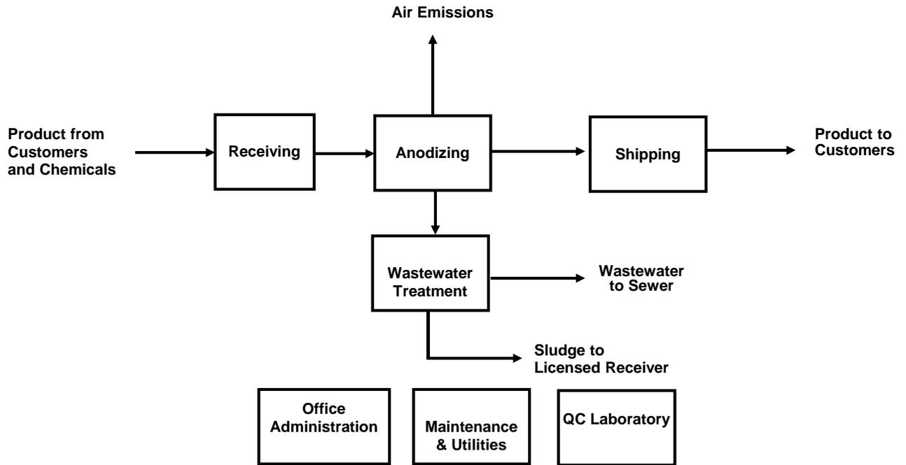
Figure 2: Anodizing Process Flow Diagram
